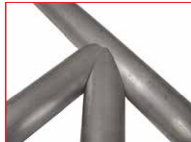
Cluster Joint Created Without Need To Remove From Vise & Reposition Tube
