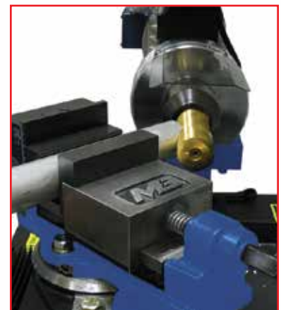
Cluster Joint Created Without Need To Remove From Vise & Reposition Tube
