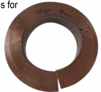
180° Bend Produced Using NEW Stretcher Die # 2700-024
